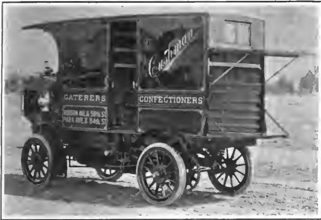
KNOX DELIVERY WAGON WITH AIR-COOLED MOTOR.
